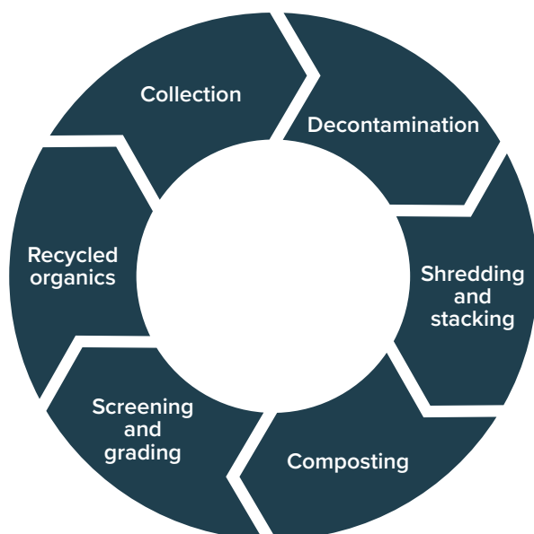
Figure 17: Solid organic waste recycling process
