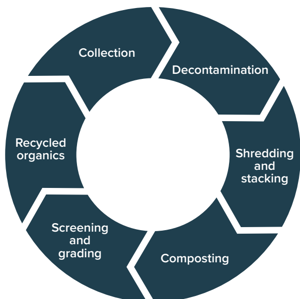
Figure 17: Solid organic waste recycling process
