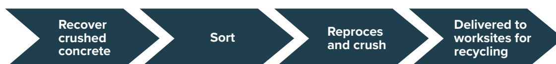
Figure 10: Material flow of crushed recycled concrete
