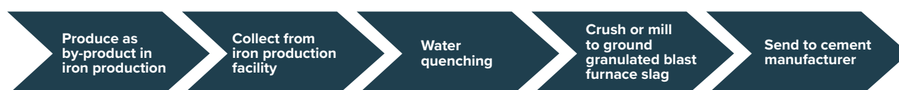
Figure 15: Processing and supply of ground granulated blast furnace slag
