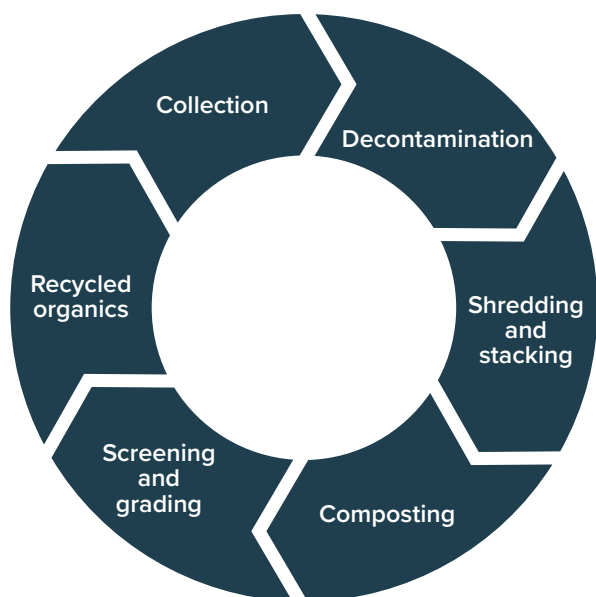
Figure 17: Solid organic waste recycling process
