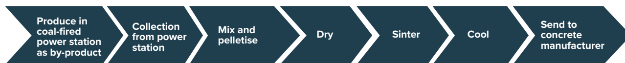
Figure 14: Production and supply of fly ash
