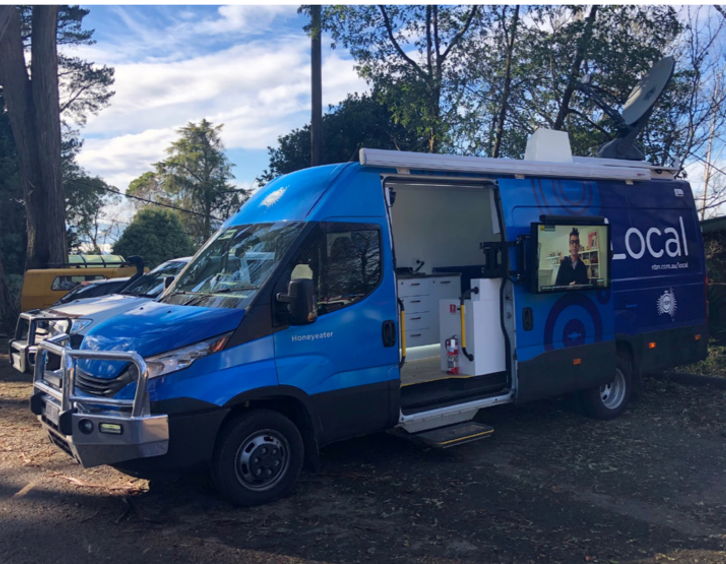
Figure 7.4: An NBN Road Muster truck provides emergency fixed wireless, wi-fi and device charging
