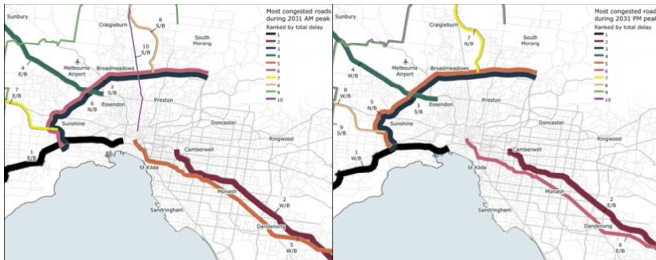
Figure 42: Melbourne’s most congested roads (total vehicle delays), 2031 AM (left) and PM (right) peak periods
