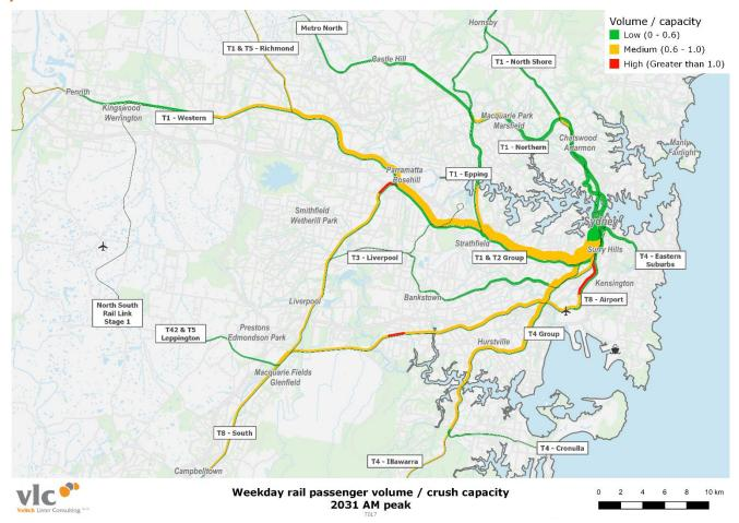
Figure 5-5 – Sydney GCCSA weekday rail passenger volume / crush capacity - 2031 1-hour AM peak
