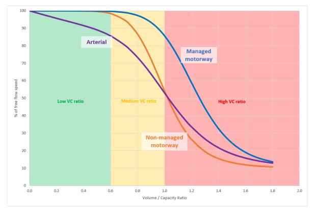
Figure 4-2 – Speed flow to volume / capacity ratio relationship
