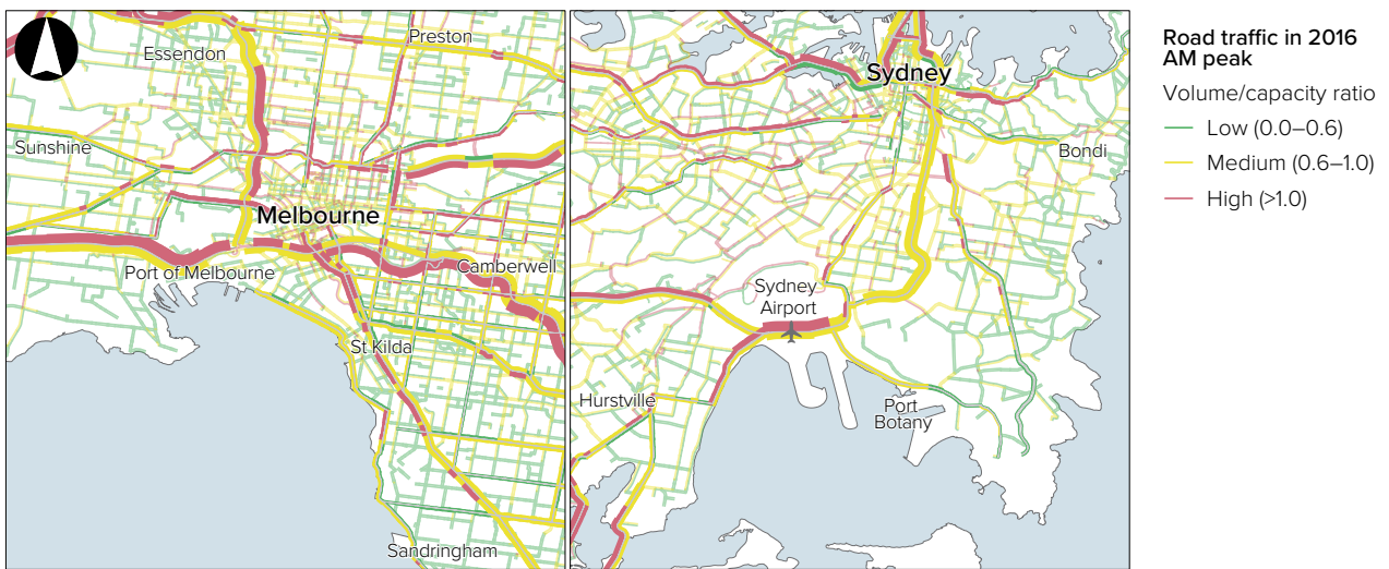
Figure 32: There is heavy congestion on key access roads to the Port of Melbourne and Port Botany
