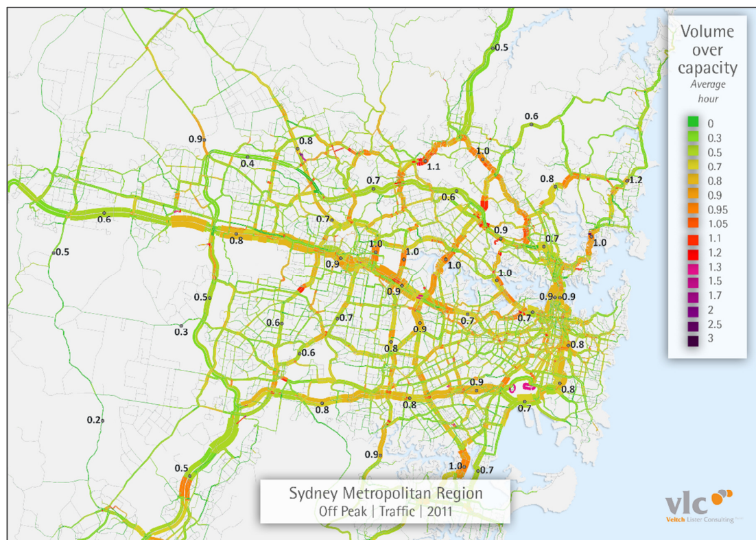
Figure 7-7: Road network volume/capacity ratios in 2011 - daytime off-peak
