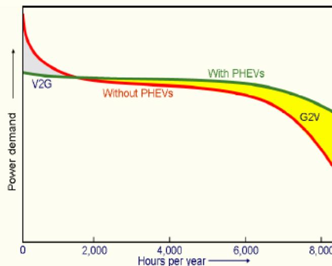
Figure 9: Impact of PHEVs on load-duration curves.
